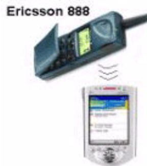
Figure 3.3 Infrared & bluetooth equipped cell phones can connect wirelessly to a mobile computer. (Source: Microsoft, 2003)
